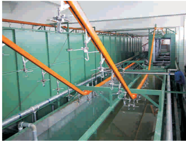
In-line dip washer with conveyORIZED system
