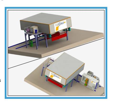
We designed, manufactured and installed this compact powder coating plant in Indonesia for the 6m aluminum profile.
