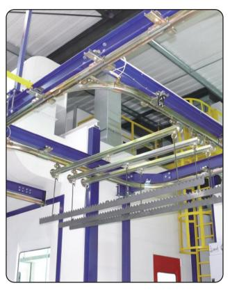
Power & free conveyor is highly automatic and integrative ,which can stop individual loads without stopping the entire production line. The main conveyor is moving continuously ,but another loading conveyor just move step by step, the output capacity can be very big if the main conveyor speed is fast ,no need to enlarge the oven size. So it takes smaller space then the common tunnel oven design.
